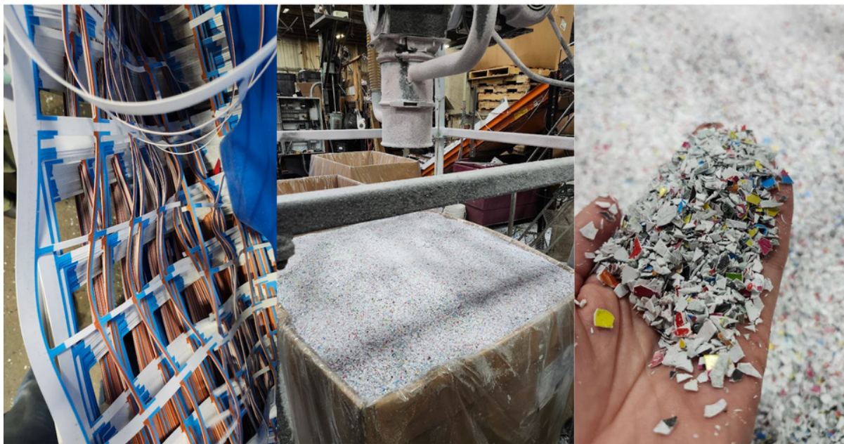
Plastic offcuts from printing operations are cut up into small pieces called regrind.
