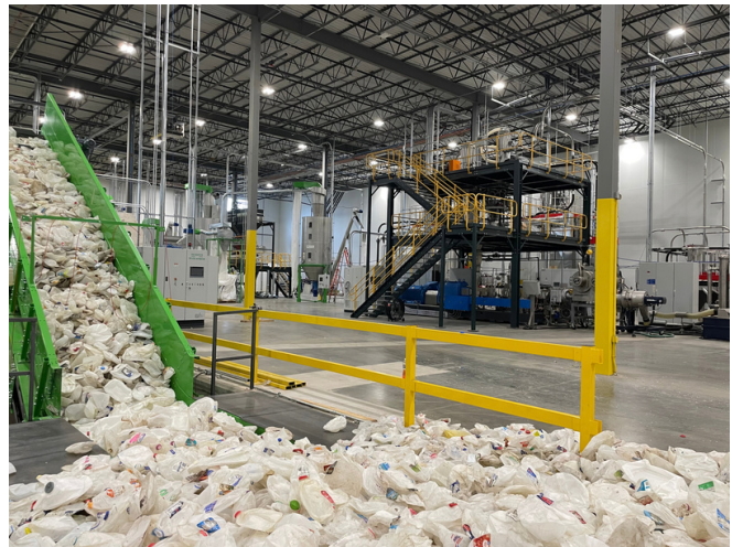
Plastic milk jugs from Eureka Recycling are sent to GDB Circular where they are recycled into pellets that can be used to make food-grade plastic containers again.
