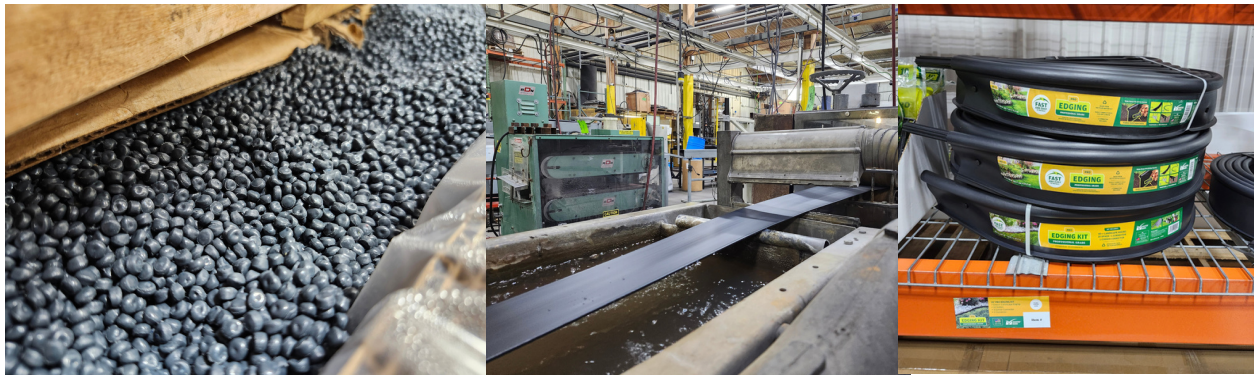
Recycled plastic pellets are melted and extruded into lawn and garden edging.
