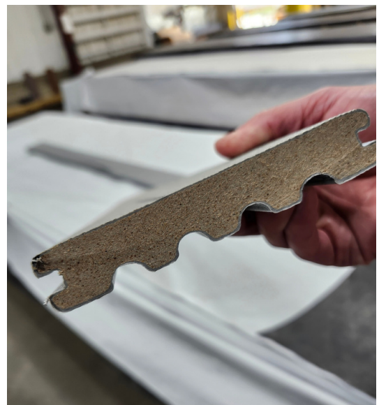
A cross-section of Avon Plastics' composite decking, showing recycled plastic and wood fibers at the core
