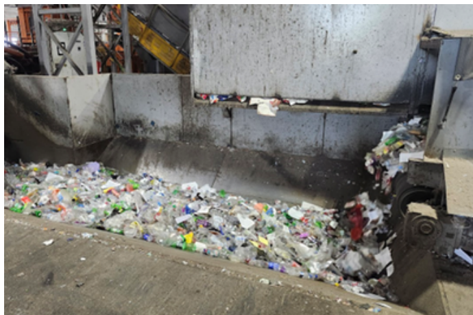
Sorted #1 (PET) plastic bottles on a conveyor belt getting ready for baling.
